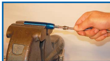
STEP 2 Flare braid using a twisting motion.
